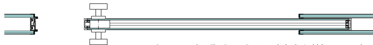
Puerta corredera Flat Door - Duo7 con hoja de 2 vidrios enmarcados Porta corredeira Flat Door - Duo7 com folha de 2 vidros encaixilhados Sliding door, Flat Door - Duo7 with double-glazed leaf, alum. frame Porte coulissante Flat Door - Duo7 avec panneau de double vitrage
